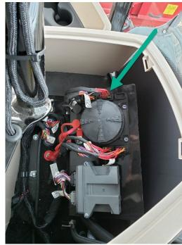
Insert the power adapter cable with the single purple wire here. This connector provides switched 12V power to the Bridge and JD components.
