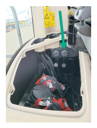
Locate the connector LCH-C225 on the forward side of the round fuse box and disconnect it.
