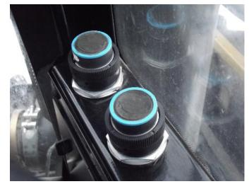
Next, connect the 31-Pin circular Deutsch end of the machine to monitor adapter to the connector that was just revealed in the previous step. Connect the other end of the adapter to the JD monitor.
