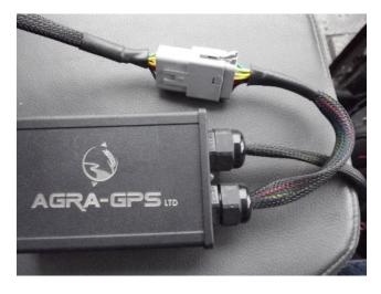
To install the machine to monitor adapter, remove the first 31-Pin circular Deutsch cap from its connector located on the left side of the cab. This will be the one located closest to the front of the machine.
