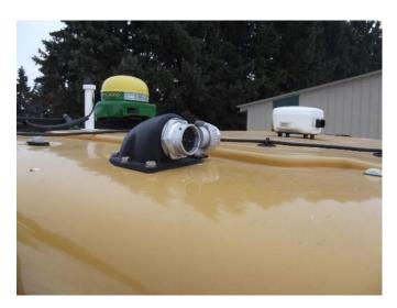
Connect the 20-Pin Amphenol end of the machine to receiver adapter to the connector mentioned in the previous step. Connect the other end of the adapter cable to the JD receiver.
