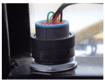
The last adapter, the machine to receiver adapter, will be connected to the 20-Pin Amphenol connector located on the roof. If this connector already has a cable connected to it, remove it.
