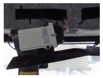
Once this panel has been removed, disconnect the existing vehicle navigation system (rectangular white box) from its wiring.
