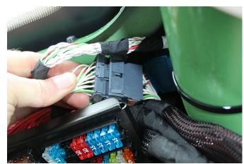
The ground wire (black) should be connected to one of the fuse panel mounts.
