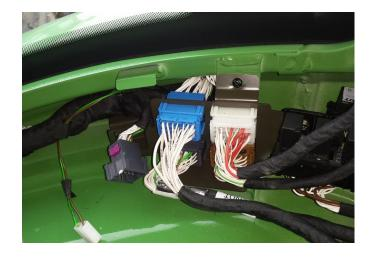
Find the gray 4214 connector and disconnect it. The Fendt-JD Bridge connects here, the other side will not be used.
