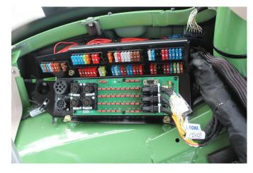
Find the gray 4214 connector and disconnect it. The Fendt-JD Bridge connects here, the other side will not be used.
