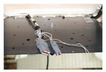
Insert the Fendt-JD bridge adapter in between the 12-pin Deutsch female plug (x4250) and its dust cap.
