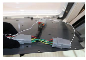
Using a process of your choosing, mount the Fendt-JD bridge to the inside of the inner metal panel. For this installation, 3M Velcro was used.
