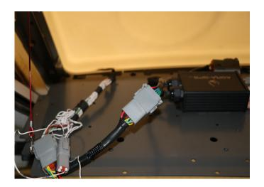
Insert the remaining 12-pin Deutsch male plug of the Fendt-JD adapter into the 12-pin Deutsch female end of the Fendt-JD bridge.
