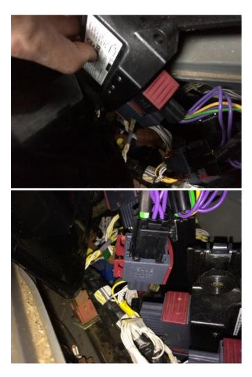
Now open the rectangle covering with the power and ISO plugs on the right side of the cab. Behind the cover you can find a couple of connectors.
