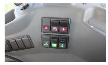
The Claas Axion autosteer activation button is located to the back right of the seat. Once the engine is started it must be activated. It will light solid green when the tractor is ready for autosteer. If the tractor was shut-off with this button in the ON position, you will have to toggle it on-off before autosteer is enabled!
