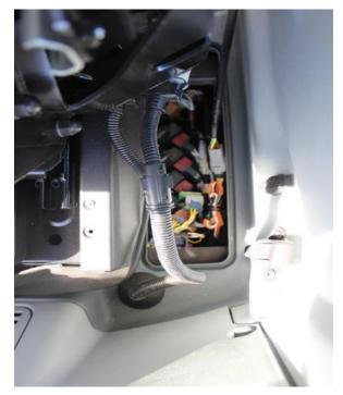
Remove the screw and put out the ATP Module. Disconnect the grey 6 Pin connector from ATP.
