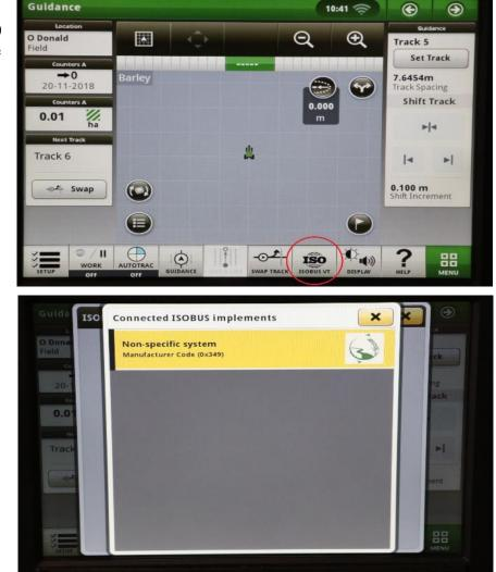
On John Deere 1800, 2600, 2630 the application will be shown in the side menu of the John Deere display. The side menu is opened by clicking the button on the bottom right of the display.
