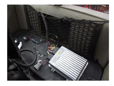
Use the red deutsch removal tool, to remove a number of connections on the 24-pin deutsch connector and re-pin them to the 40-pin deutsch on the same cable.
