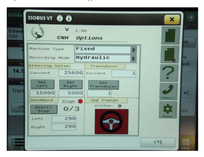
**Section – Steering Valve:** Allows the user to set the left and right max of the CNH machine. To calibrate, steer as far left as possible and press, "Set Left". Then, steer as far right as possible and press, "Set Right".
