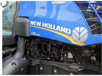
Now take the  $3^{rd}$  adaper and connect the portA (X-295) + portB (X-433A) connectors from the machine to the John Deere GPS receiver (here a SF6000). The receiver must be mounted at the front of the roof!
