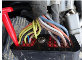
Use the  $2^{nd}$  adapter which has the black 40-pin deutsch connector, and the long cable to the 2-pin deutsch (DT).
