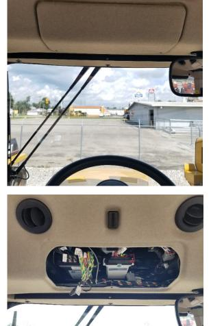
Disconnect the plug from the existing controller.
