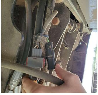
Take the terminator plug back into the cab and connect it to the 3 pin Deutsch plug coming off the 12 pin Deutsch plug that connects to the bridge.
