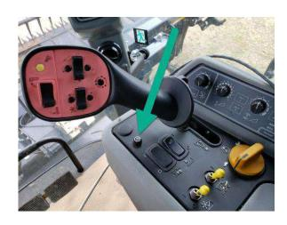
In order for yield and moisture to be displayed on the JD Monitor, a task must be started on the AGCO monitor in the machine.
