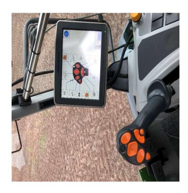
Also the Amazone ISO application to control the sprayer should load.
