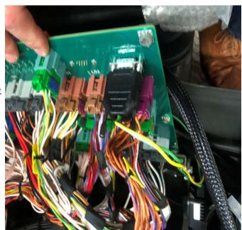
Now connect the 9-Pin ISO-BUS incab connector of the provided adapter harness to one of the machine.incab ports.
