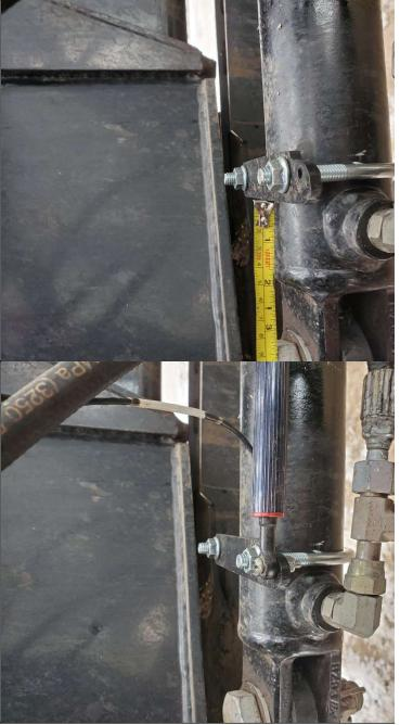
Mount the sensor body to the top of the plate. The sensor must be mounted on the top of the plate.
