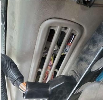
Find the connector labelled C602 behind the panel. Open it and insert the 12-pin DTM connectors of the provided AgraGPS harness.
