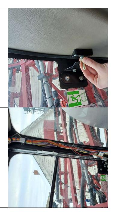
Remove the plastic cover revealing the post cabling.
