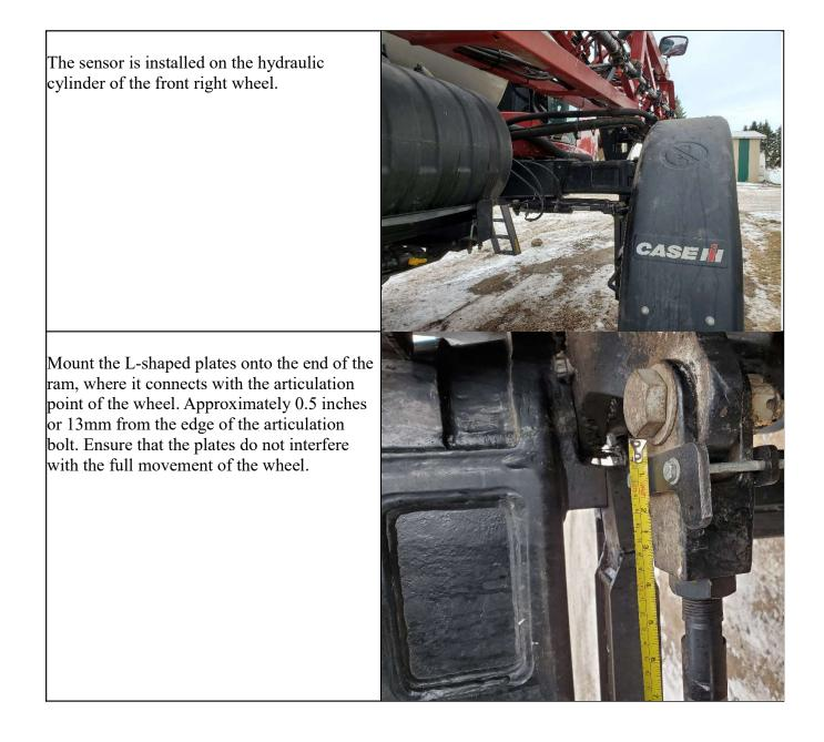
Mount the U-Bolt plate at the other end of the hydraulic cylinder, just past the end-port connection. Approximately 2 inches or 50mm from the end of the cylinder.
