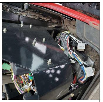
Using the included removal tool, remove the wire in pin 3 of the 24-pin connector. Once removed, push the pin into pin 7 of the 40-pin connector.
