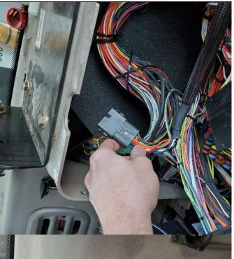
The "vent" behind the seat can be removed to assist in feeding the cable through to the corner post.
