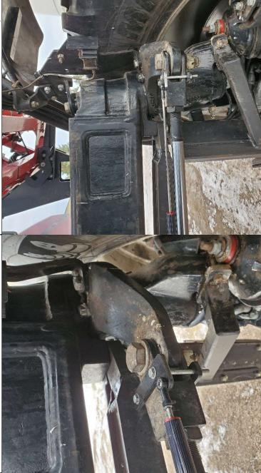
Next turn the wheel all the way to the right, ensure that the sensor can be secured without hitting the sensor end stop.
