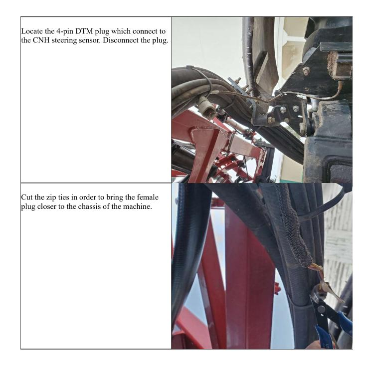
Bring the plug closer to the chassis of the machine and replace the cut zip ties.
