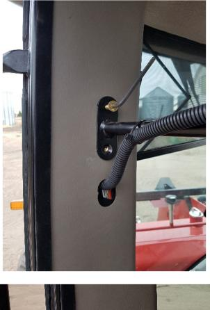
Now remove the door latch which still holds the plastic cover in its place.
