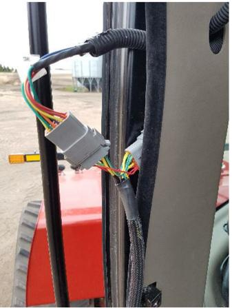
Now run the the display cable though the oval opening.
