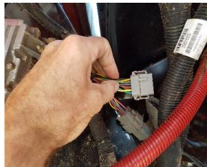
The 2<sup>nd</sup> part of the adapter inserts into the 12-pin deutsch conenctor going to the seat.
