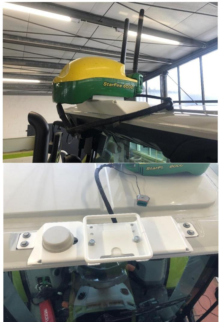
**Step 4: Once the receiver is installed, check the settings for the JD Receiver in the display! Also make sure you do a TCM calibration.**
