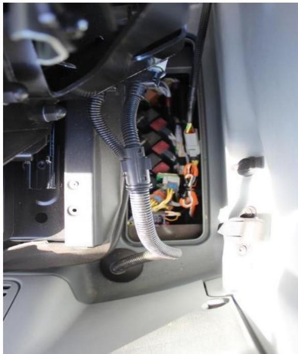
Now open the rectangle covering with the power and ISO plugs on the right side of the cab. Behind the cover you can find a couple of connectors.
