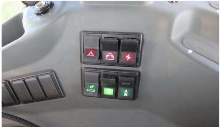
The Claas Axion autosteer activation button is located to the back right of the seat. Once the engine is started it must be activated. It will light solid green when the tractor is ready for autosteer. If the tractor was shut-off with this button in the ON position, you will have to toggle it on-off before autosteer is enabled!
