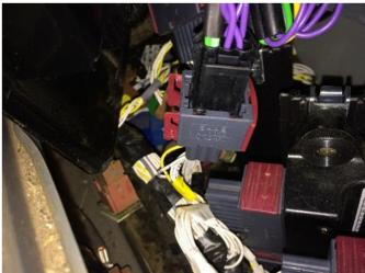
Now open the rectangle covering with the power and ISO plugs on the right side of the cab. Behind the cover you can find a couple of connectors.
