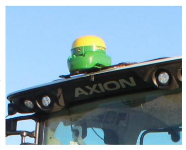
Step 4: Once the receiver is installed, check the settings for the JD Receiver in the display! Also make sure you do a TCM calibration.
