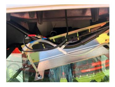
After the cable is out of the roof and the plastic covers are mounted again reassemble the 12-pin deutsch connector.
