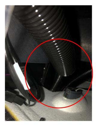
Remove the wedge in the 12-pin deutsch connector and carefully pull the cables backwards out of the connector. You will need a small flat screw driver to release the plastic clamps inside the connector. MAKE A NOTE OF THE PIN/CABLE LAYOUT BEFORE YOU REMOVE THE CABLES! Disconnecting the deutsch connector allows you to run the cable behind the plastic and through the cable canal. May put some isolation tape around it to protect the pins!
