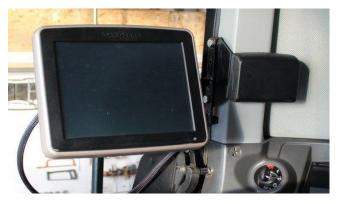
Another option is to use two 1.5-inch RAM mount balls (RAM-202U) and a 4-inch double socket arm (RAM-201U). You can find this under the order number Order the D-JD-RAM together with the display mounting plate from Agra-GPS.
