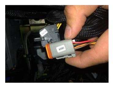
Now connect the grey 6Pin Deutsch connector of the adapter.
