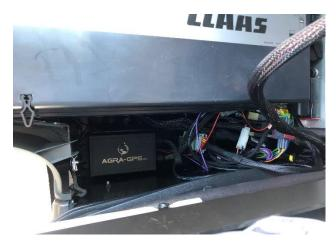
Connect the 6Pin ends of the adapter with the ATP Module which is located on the right side next tot he driver seat.
