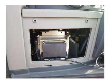
You will find 6 connectors. 4 of which are 2-pin deutsch, the other 2 are the black 3pin connectors. In the picture they are already connected to the Horsch-JD bridge adaptor cable.
