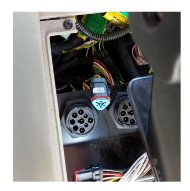
Remove the cover at the left side where the 3-Pin power socket is located.
