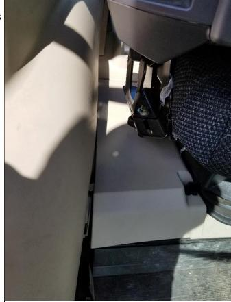
Locate the X230 connector, open the connector, and connect both ends of the matching Agra-GPS adapter to the now open ends.
