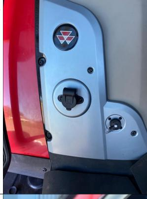
Locate the X150 connector, open the connector, and connect both ends of the matching Agra-GPS adapter to the now open ends.
