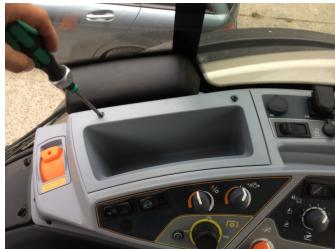
The connector X11C behind the panel shown in the picture.
