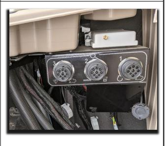
Then, insert the 12-pin Deustch 'in-between' connectors of the GleanerS9-JD adapter in between the Deustch connectors on the cable that is routed through the floor located just to the right of the driver's seat. These connectors may need to be exposed, as occasionally they are tucked into the hole they are routed through.
