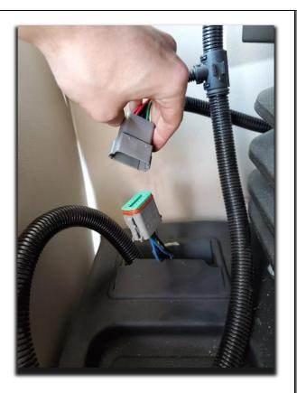
Connect the final end of the GleanerS9-JD Adapter, the 12-pin male Deutsch connector, into the 12-pin female Deutsch connector of the GleanerS9-JD bridge.
