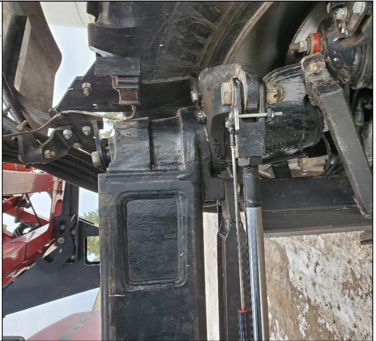
Next turn the wheel all the way to the right, ensure that the sensor can be secured without hitting the sensor end stop.
