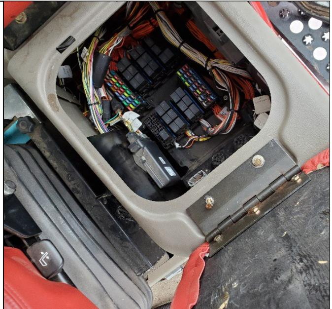
Remove the plastic cover that was under the buddy seat, there are bolts under the rubber floor mat that must be removed.
