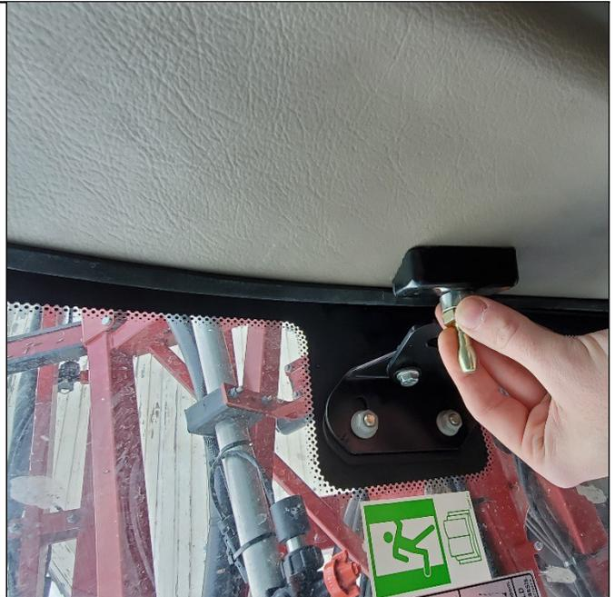
Remove the plastic cover revealing the post cabling.
