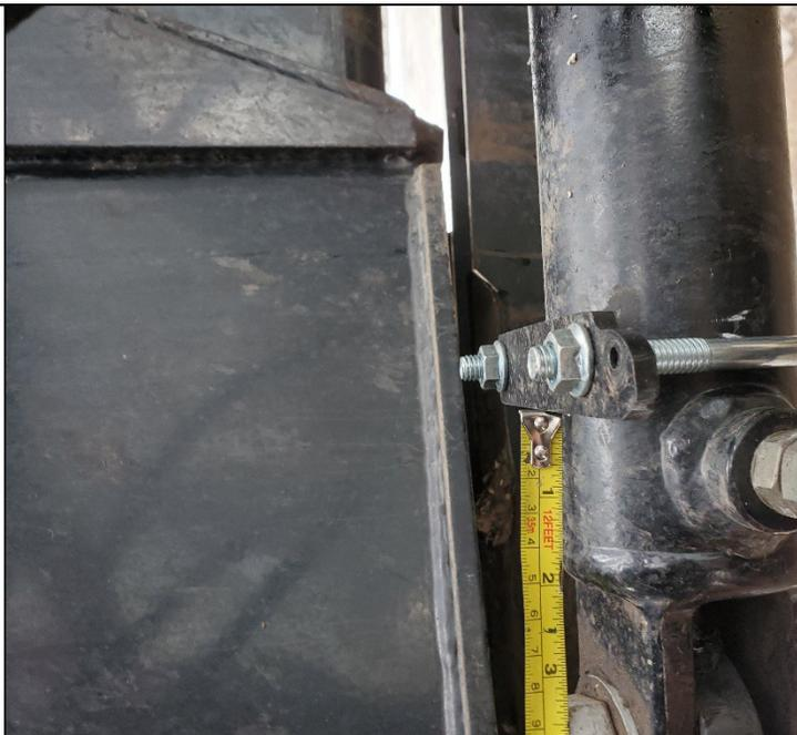
Mount the sensor body to the top of the plate. The sensor must be mounted on the top of the plate.
