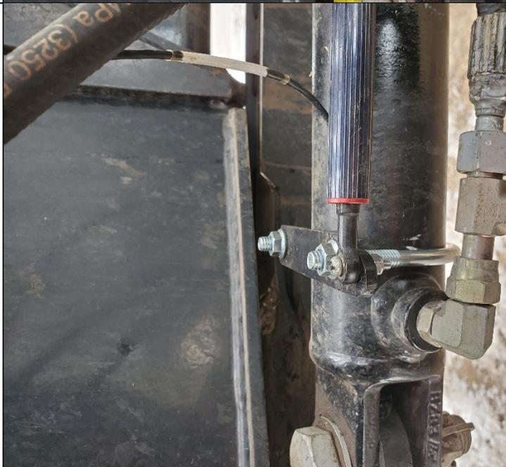
While the other end of the sensor is not secure, turn the wheel all the way to the left, ensure that the sensor can still be secured without exceeding its movement range.
