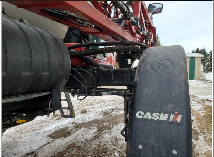
Mount the L-shaped plates onto the end of the ram, where it connects with the articulation point of the wheel. Approximately 0.5 inches or 13mm from the edge of the articulation bolt. Ensure that the plates do not interfere with the full movement of the wheel.
