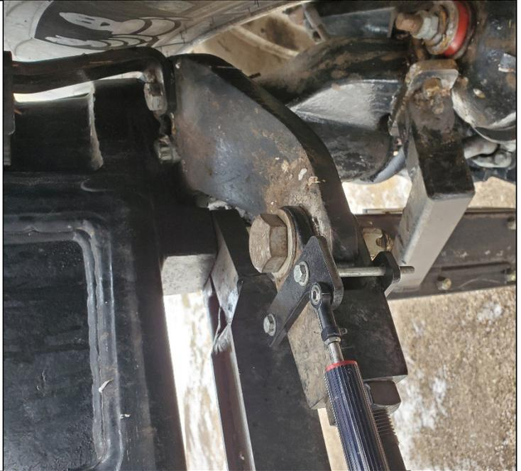
Locate the 4-pin DTM plug which connect to the CNH steering sensor. Disconnect the plug.
