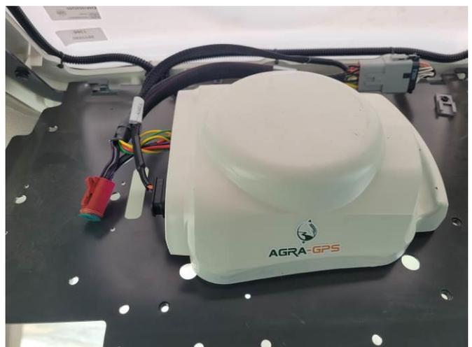
The CRG contains an RTK receiver which, like any RTK receiver, requires RTCM correction data. To achieve this, you may use an Internet-based NTRIP server.
