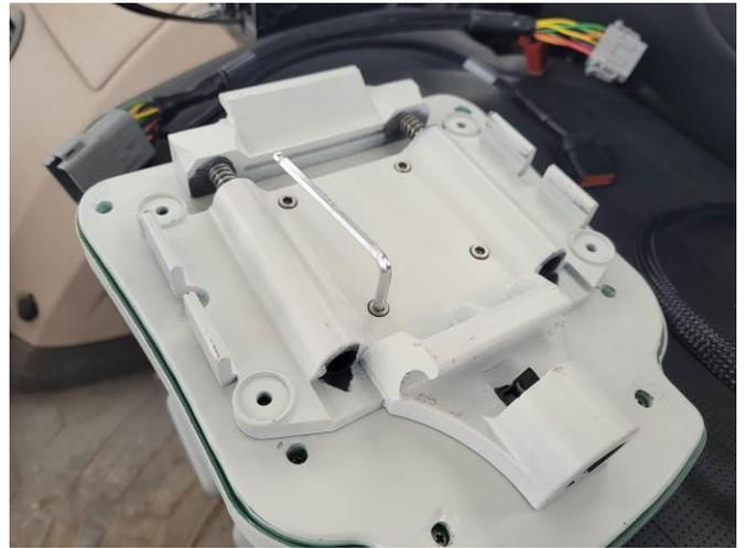
The JD bracket is only needed when you use the CRG as a receiver on a John Deere machine and mount. For the Fendt installation it is not required.
