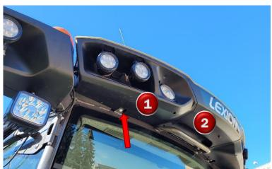
Install with bracket <u>square</u> to machine and flush to the front of the eyebrow. Drill through plastic and install bolts with locking nuts.
