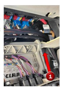
3) Push a thin stick (roughly 4 feet long) from the outside into the cab. Tape the receiver connector to the stick and pull through to the outside.
