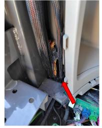
The monitor cable requires routing up to the monitor mount. Route through one of the relief holes at the bottom front of the window. It is possible (barely) to force the monitor plug through the hole without damage. Route the cable up and underneath the rubber weatherstripping to the monitor mount.
