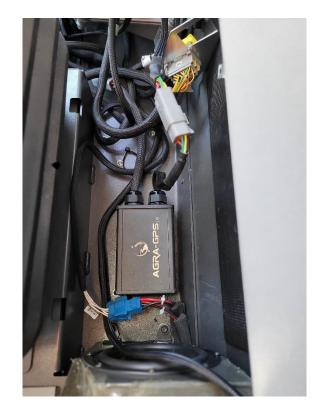
Locate the X485 connector below the operator seat (right hand side). It will be attached to termination resistor labelled as XR014.3 (connected through plug X48T). Remove this from the X485 connector, and connect it to the other side of the Bridge.
