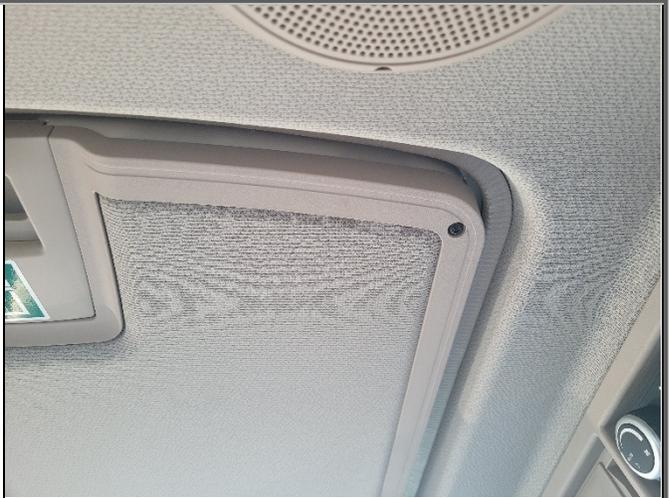
To access the connector for steering, you need to remove all the bolts securing the inner panel, allowing it to swing down.
