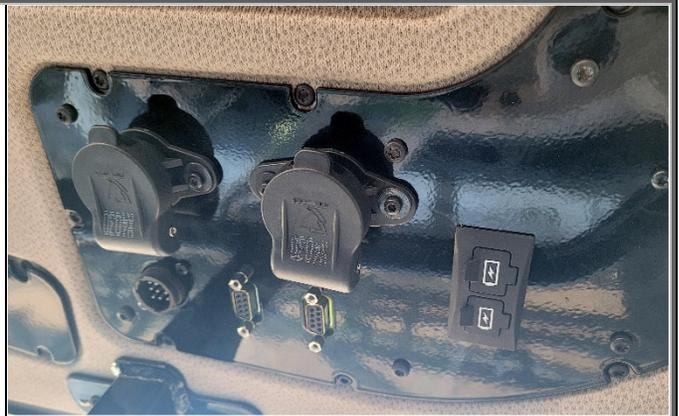
Insert the circular 9-pin female end of the monitor to machine adapter into the 9-pin male ISO in-cab connector.
