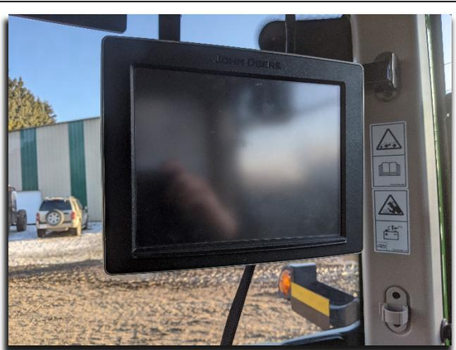
For a Rogator sprayer you want to use a 4gen JD display as the 3gen displays are limited to 16 sections!!
