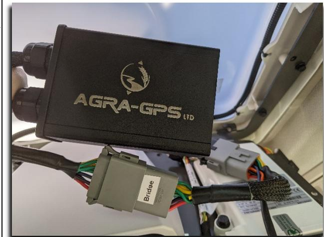
Next, insert the 12-pin Deutsch female end of the bridge to GPS adapter cable (12-pin Deutsch female to 12-pin Deutsch male cable) into the Agra-GPS AGCO-JD Bridge. Route the 12-pin Deutsch male end of the same cable to the roof outside of the machine and connect it to your JD GPS.
