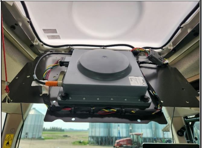
Locate the X21 connector (shown right) and disconnect the female connector from the male connector.
