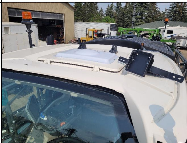
It is easier to work with the latches with the roof panel opened as some pressure is removed from the gas filled cylinders.
