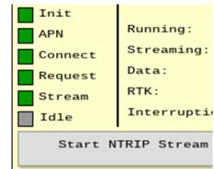
When the Stream indicator shows green, you are streaming! With a good satellite signal, you should now have RTK Fix quality precision. Go to the CRG Diagnostics page to verify that all RTK settings show green. Streaming rates that successfully achieve RTK Fix can typically measure between 10 to 40 kB per minute, depending on how the base station’s output rate is configured.
