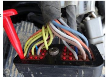
Use the 2<sup>nd</sup> adapter which has the black 40-pin deutsch connector, and the long cable to the 2-pin deutsch (DT).
