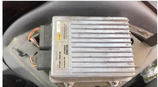
Move a wire from the 24-pin connector and re-pin it to the 40-pin on the same cable.
