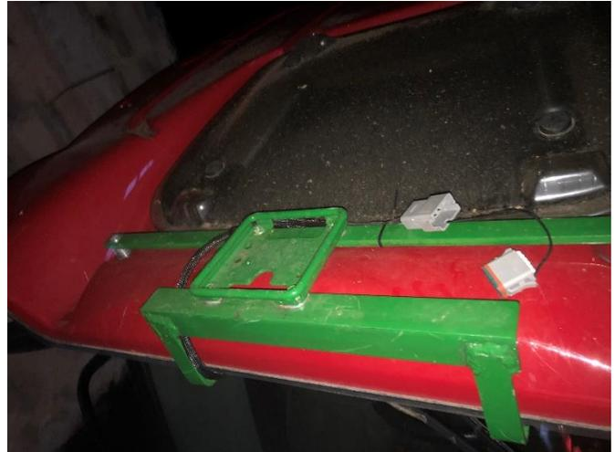
Also run the harness from the to the John Deere display (here a 2630).
