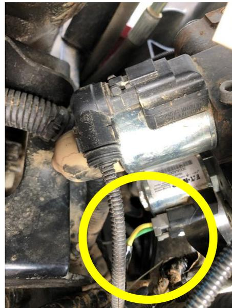
Use the 2<sup>nd</sup> adapter which has the grey 12 Pin Deutsch connector and at the other end the ISO in-cab connector and the Diagnostic connector.
