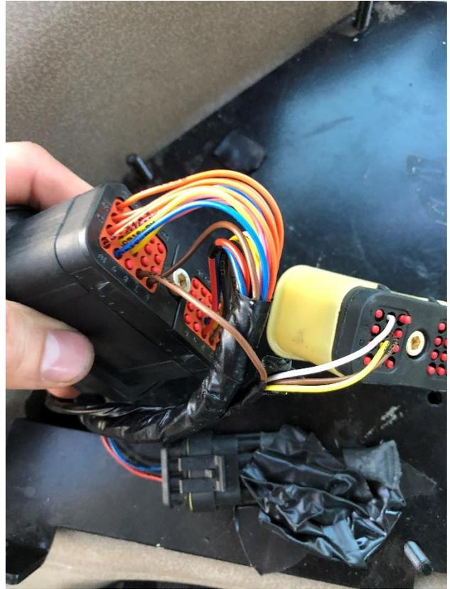
Run the 2-pin deutsch under the floor in the inside cab to the front where the clutch is located. There you can find an outlet with a rubber pad.
