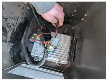
Use the red Deutsch removal tool to remove the wire in pin 3 from of the 24-pin connector, then insert it into pin 7 on the 40-pin connector.
