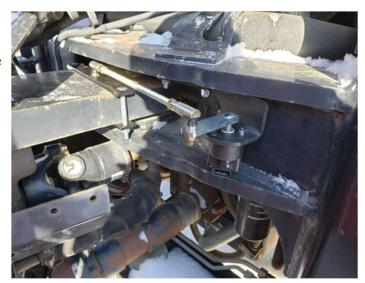
Mount the 2 flat bars as close as possible to the turning point.
