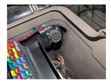
Route the 8-pin and 40-pin cable behind the seat into the area underneath the buddy seat.
