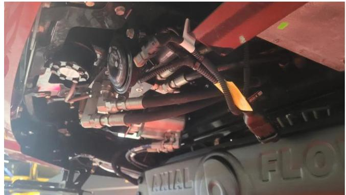
Connect to the X1214P near the steering valve.
