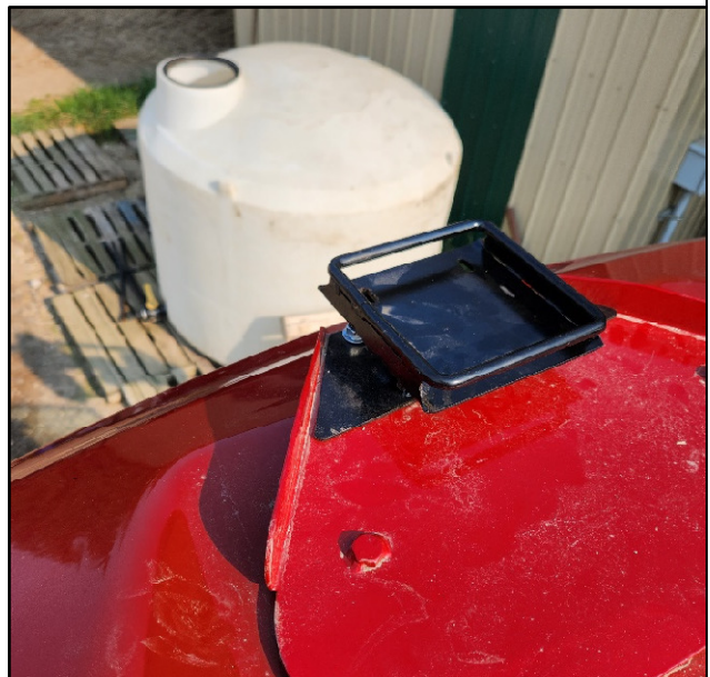
Figure 4-D – GPS Receiver Bracket Installed
