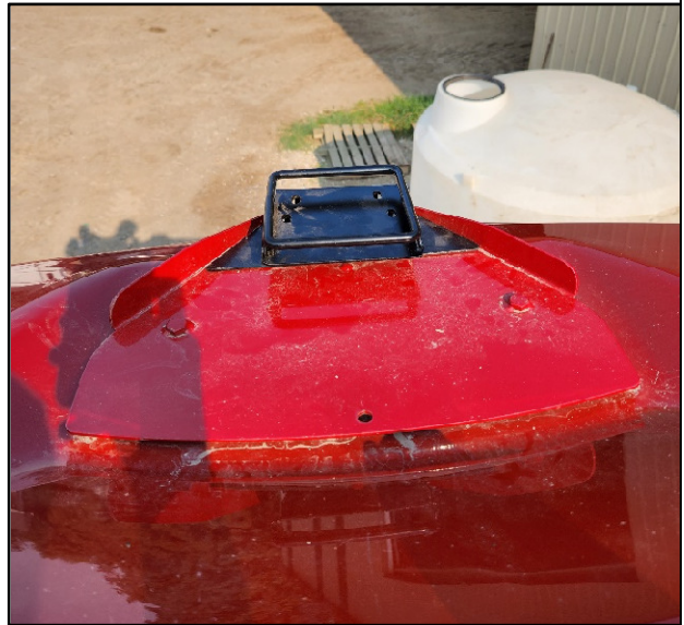
Figure 4-C – GPS Receiver Bracket Installed
