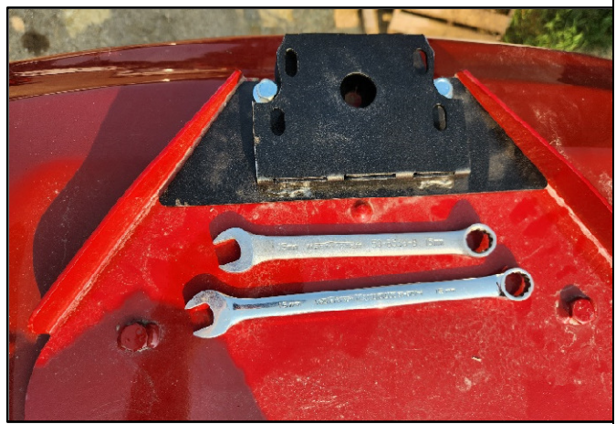
Figure 4-A – Installation of Base GPS Receiver Bracket
