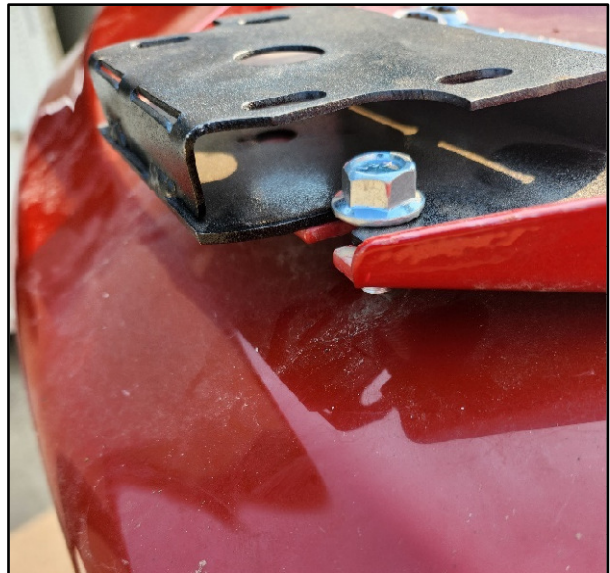
Figure 4-B – Installation of Base GPS Receiver Bracket
