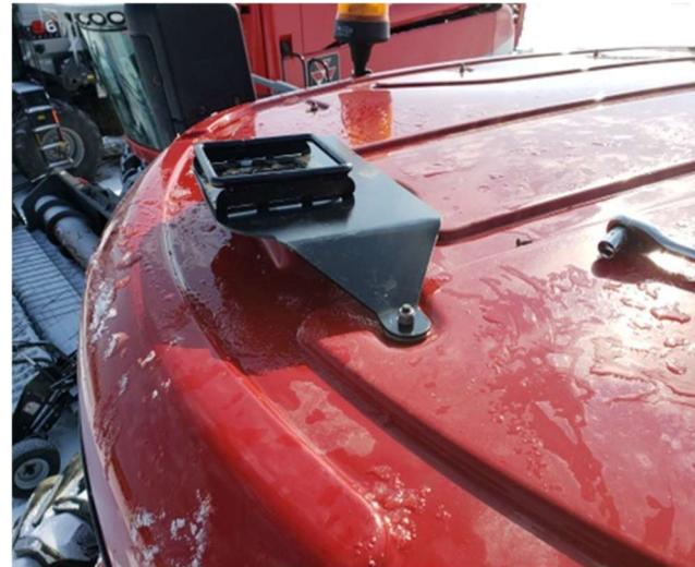
The JD mount can easily be bolted to the metal bracket provided on the roof of the CNH Quadtrac.
