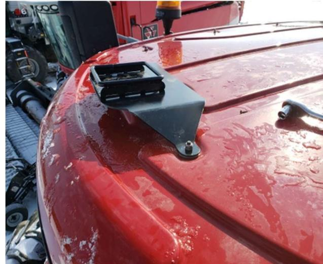
Using the short 12-pin adapter cable, the JD receiver is connected to the 12-pin Deutsch in the CNH tractor roof.
