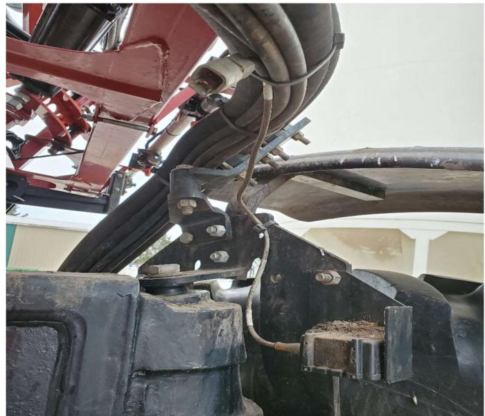
Cut the zip ties in order to bring the female plug closer to the chassis of the machine.
