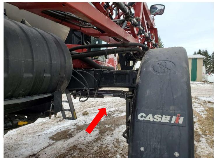
Use supplied bolts to install L bracket on outside end of the right-side steering cylinder. Place the L bracket on the front.
