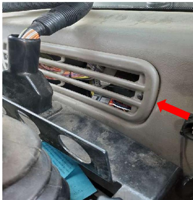
Find the connector labelled C602 behind the panel. Open it and insert the 12-pin DTM connectors of the provided AgraGPS harness.
