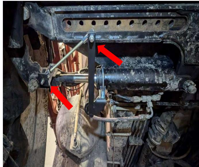
Locate the 4-pin DTM plug which connect to the CNH steering sensor. Disconnect the plug.
