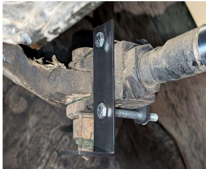
Place the clamp on the steering cylinder tube, then install the sensor housing bracket on the back side.
