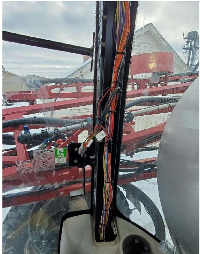
Then connect the 12-pin black mini Deutsch and the 12 pin grey mini Deutsch plugs to the bridge. The bridge can be left behind the plastic cover below the pillar post cover. It can be easily accessed while the side door is open.
