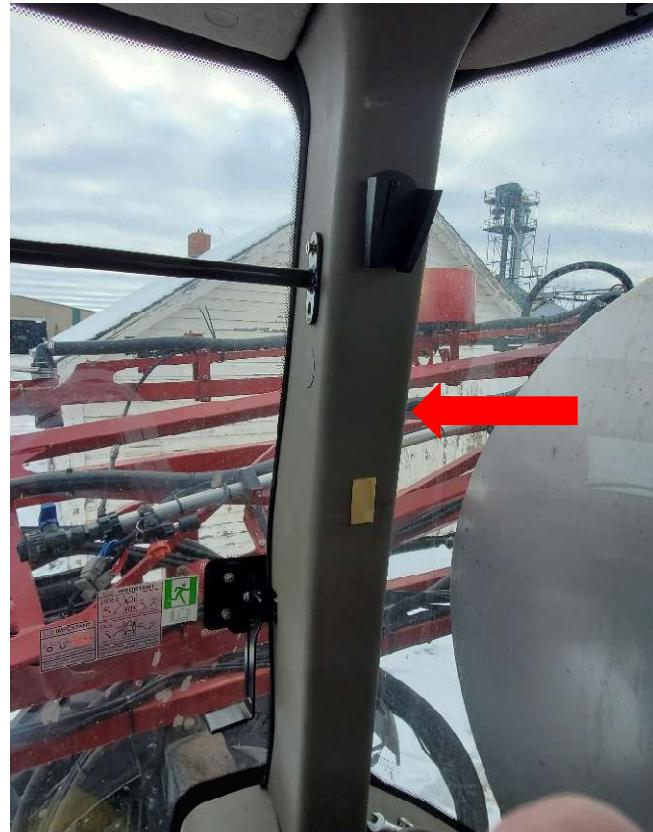
Remove the bolts holding the crossbar to the corner post.
