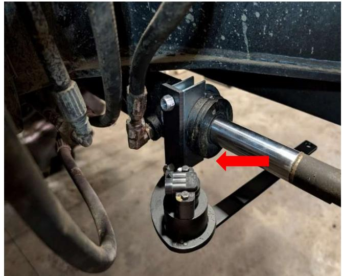
Install threaded rod with ball joints to connect both brackets.
