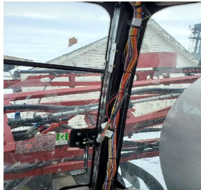
The 40-pin adapter connector must be fed through to the buddy seat (fuse panel) area. It can be fed through from below the right corner post, behind the plastic behind the seat, and through to the 40-pin machine connector at the fuse panel.
