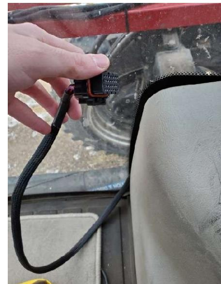
Then connect the harness to the monitor. The monitor can be mounted using RAM components, which can be ordered from Agra-GPS.
