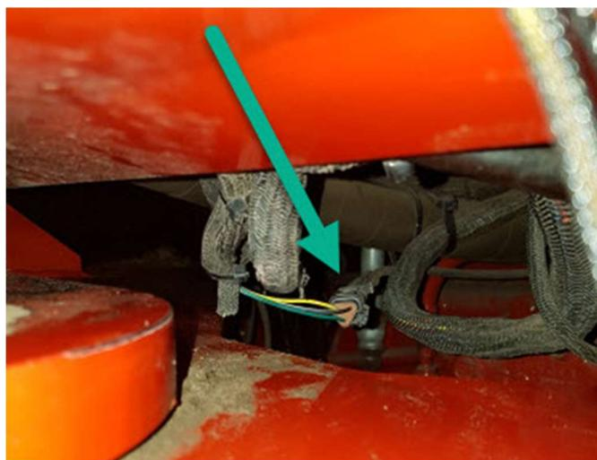
Find the Sauer Danfoss valve with its 4-pin valve connection and the 3-pin transducer connection.
