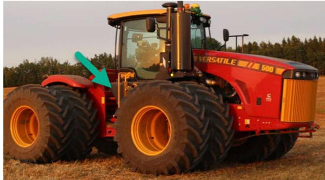
Find the green 12-pin Deutsch under the cab. It is located in the center back of the cab.
