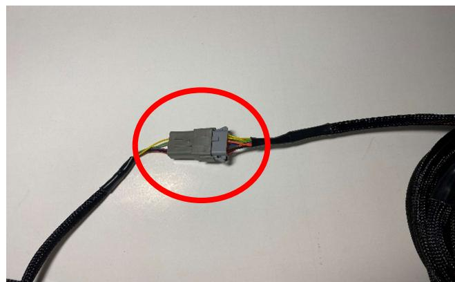
The black connector on the JD-12 harness will connect to the monitor. The grey 12-pin connector on the JD-12 will connect to the outside receiver.
