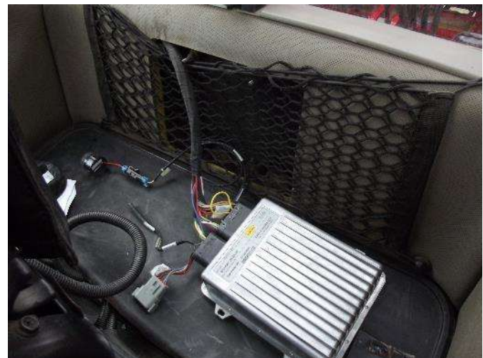
Nav controller behind interior plate
