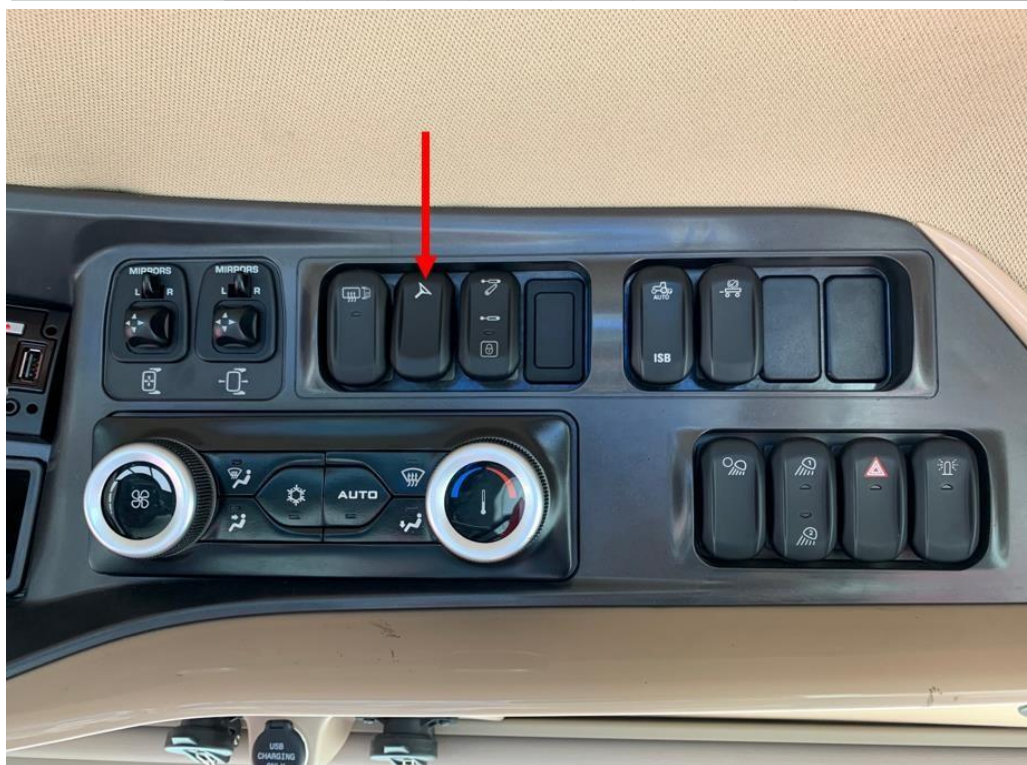
Headliner Road Switch
