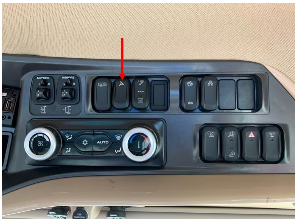
Headliner Road Switch
